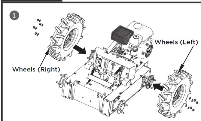
Put a pair of wheels onto the rear wheel axles and make sure the tyre valve is facing outwards. Slide the four bolts off each wheel axle through the hoels in wheels and secure them with M12 nuts and washers.
