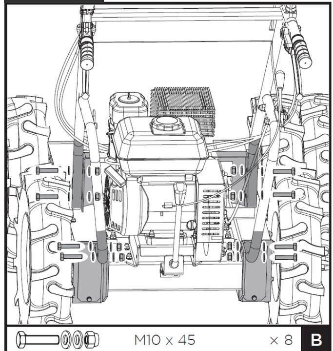
Mount the handle frame assembly to the chassis and secure it with M10x45 bolts, washers and nuts.
