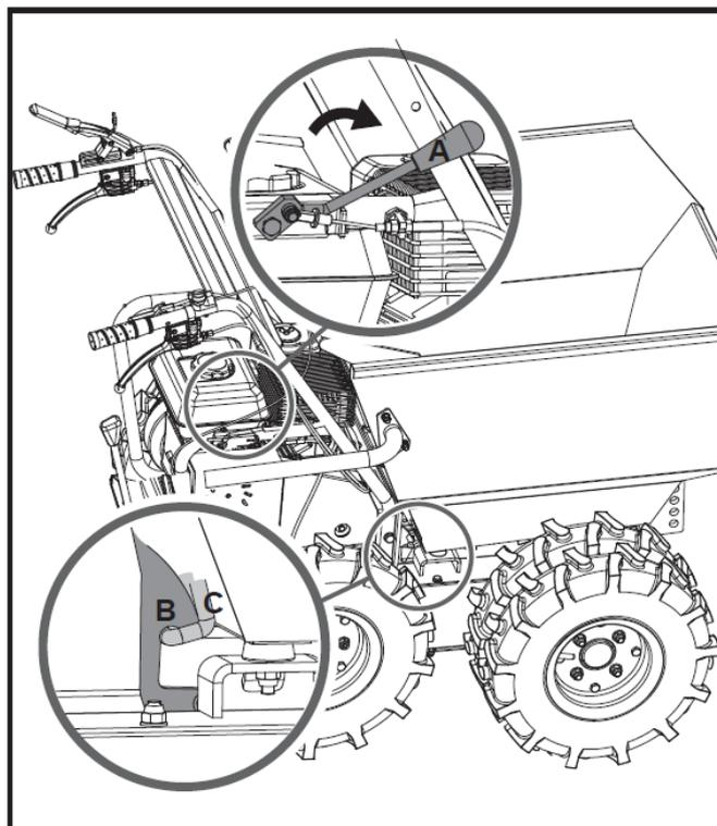
**!** Before you start to use the dumper, please check the dump box to make sure it is locked as shown in the diagram below.
