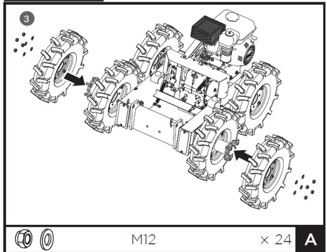
Mount the last pair of wheels on outer side of the fixed front wheels to the welded flange plates by M12 nuts and washers.
