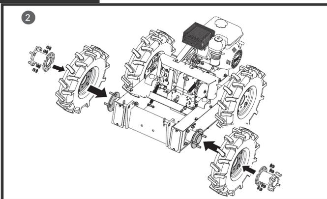
Attach another pair of wheels to the front wheel axles. Connect the welded flange plates to both wheels by the bolts of wheel axles and secure them together with M12 nuts and washers.
