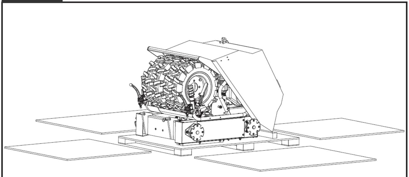
Remove all the plywood plates, and remove all the loose parts on the bottom pallets.
