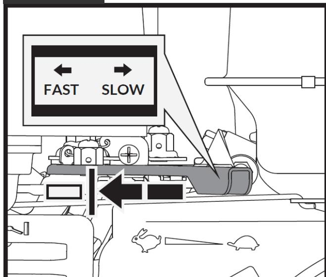
Move the throttle lever slightly to the FAST speed.
