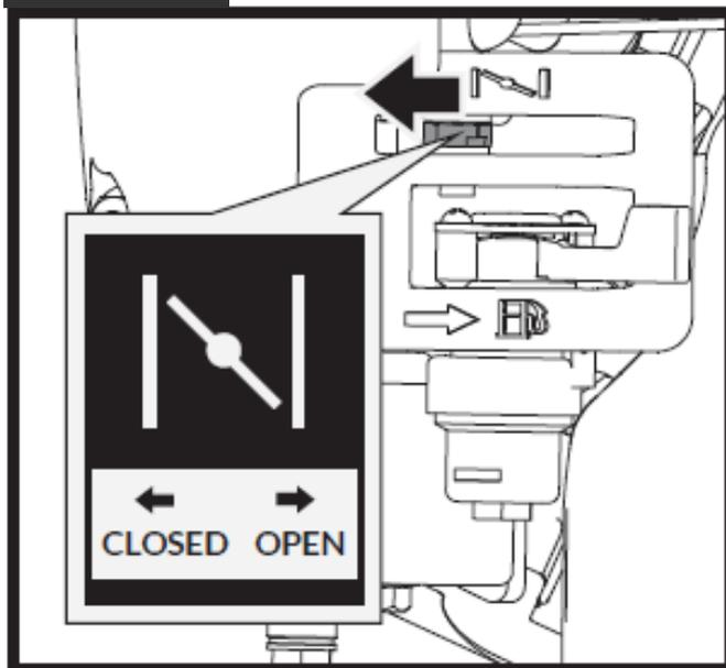
Move the choke lever to the CLOSED position. If the engine is hot, closing the choke is not necessary.
